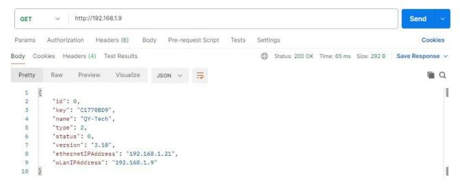
Host name access. The default host name of the device is QY-Tech. You can modify the device host name (4.2 interface). Note: When multiple hosts with the same name are registered in DNS, the device registered first will generally be accessed, and the high network segment may not be able to access the DNS of the low network segment.
